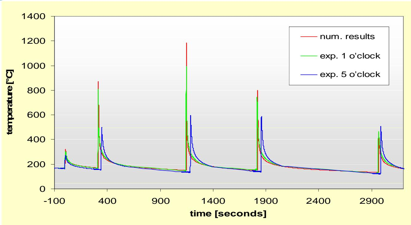
Results for point B (1mm of the surface) shown on the finite element mesh
