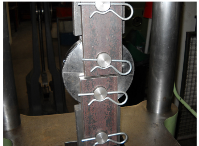
Fig. 9. Split ring test assembly.
