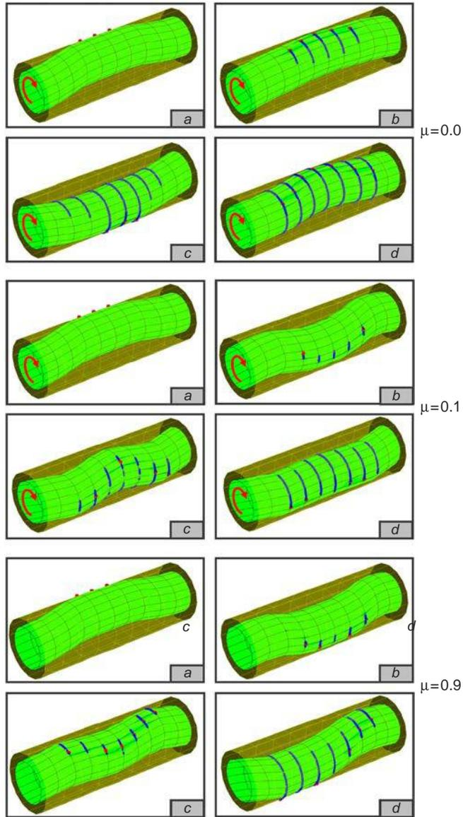
**Notes:** In blue we show the time evolution of the contact points and in red the location of the contact point at the time of the drawn configuration. It is indicated with “a,b,c and d” four consecutive configurations
