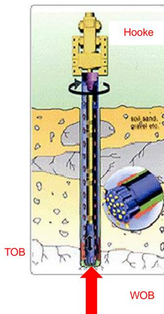
**Figure 9.** Schematic representation of TOB-WOB and Hook
