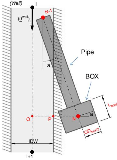
**Figure 4.** Geometry of the contact pipe/well (in this case the contact algorithm needs to correct the geometry and the kinematics)
