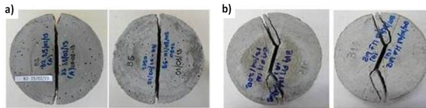
**Figure 5.** Experimental results for the Brazilian test with a slot for mode I. a)  $\alpha = 0^\circ$ . b)  $\alpha = 28^\circ$ .
