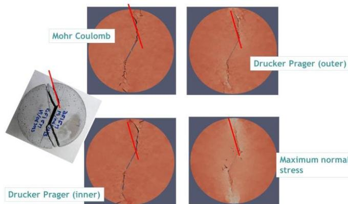
**Figure 6.** Brazilian Test with a slot: experimental vs. numerical results
