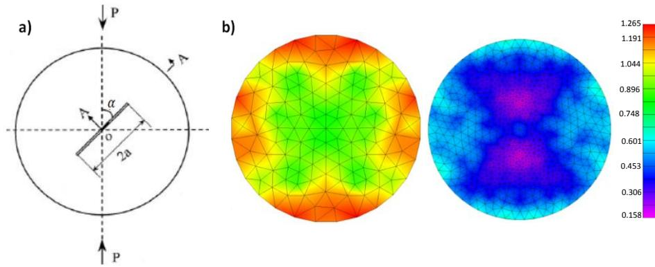
**Figure 2.** a) Cylindrical sample with a through slot [15]. b) Meshes used to model the notch Brazilian Test. The contour map indicates the mesh quality factor  $l/l_c$  (see Eq. (4) for more details).
