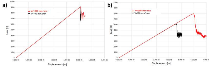
**Figure 3.** Results for the Brazilian test with a slot. **a)** Coarse mesh results. The black line represents the response of the specimen with a load velocity 100 mm/s. The red line represents the response of the specimen with a load velocity 1000 mm/s. **b)** Finer mesh results for 100 mm/s (red) and for 1000 mm/s (black).
