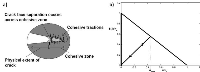
Figure 1. a) Fracture propagation. b) Cohesive law
