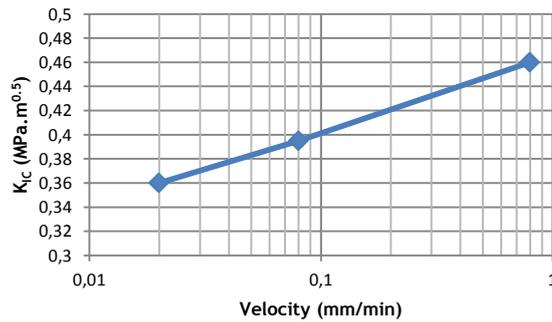
**Figure 4.** Variation of the fracture toughness for the synthetic samples as function of the loading velocity.
