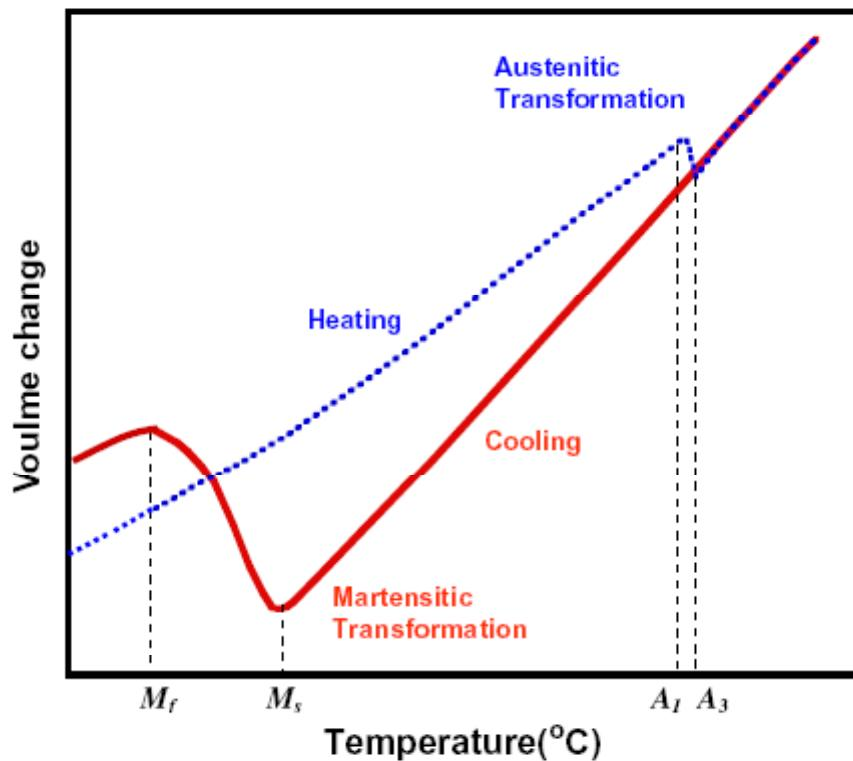
Fig. 4. Schematic diagram of volume change due to phase transformation.
