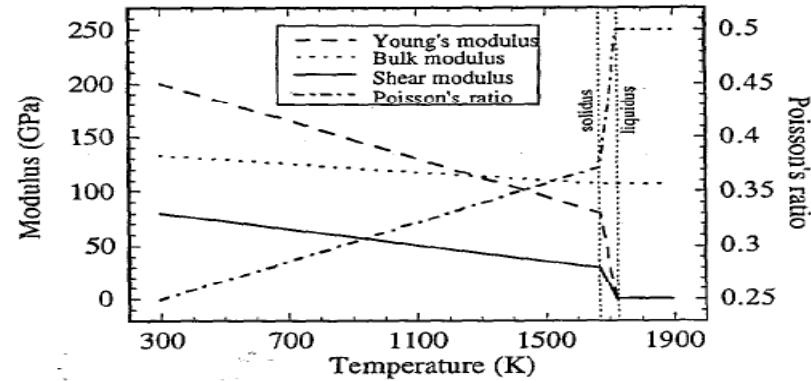
Figure 4. Elastic properties of 304L stainless steel used in mechanical finite element analyses.
