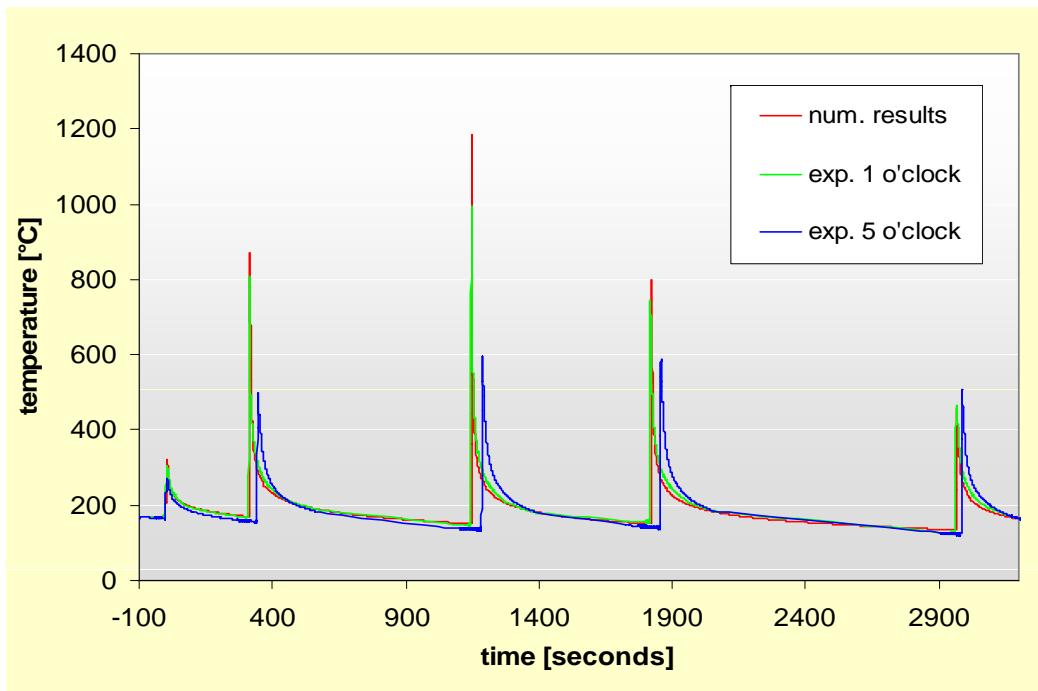
Results for point B (1mm from the surface) shown on the finite element mesh
