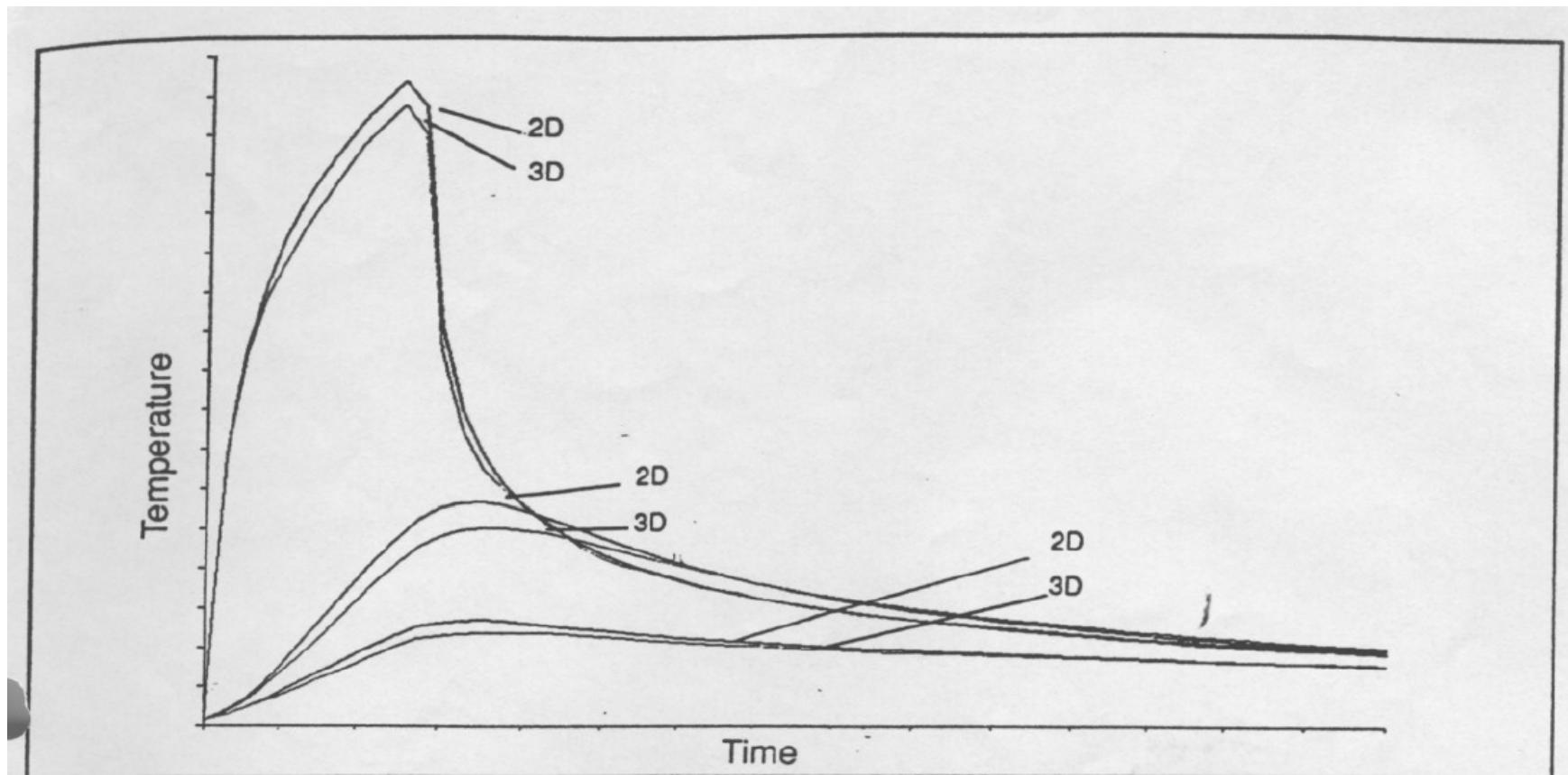
Figura 2: Thermal cycles predicted with 2D and 3D FEM models at points A,B and C (see Fig.3) during a single pass weldment.
