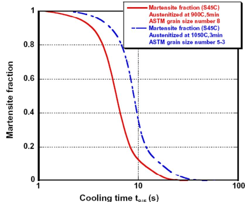
Fig. 6. Martensite fraction as a function of cooling time  $t_{8/5}$  for S45C steel.
