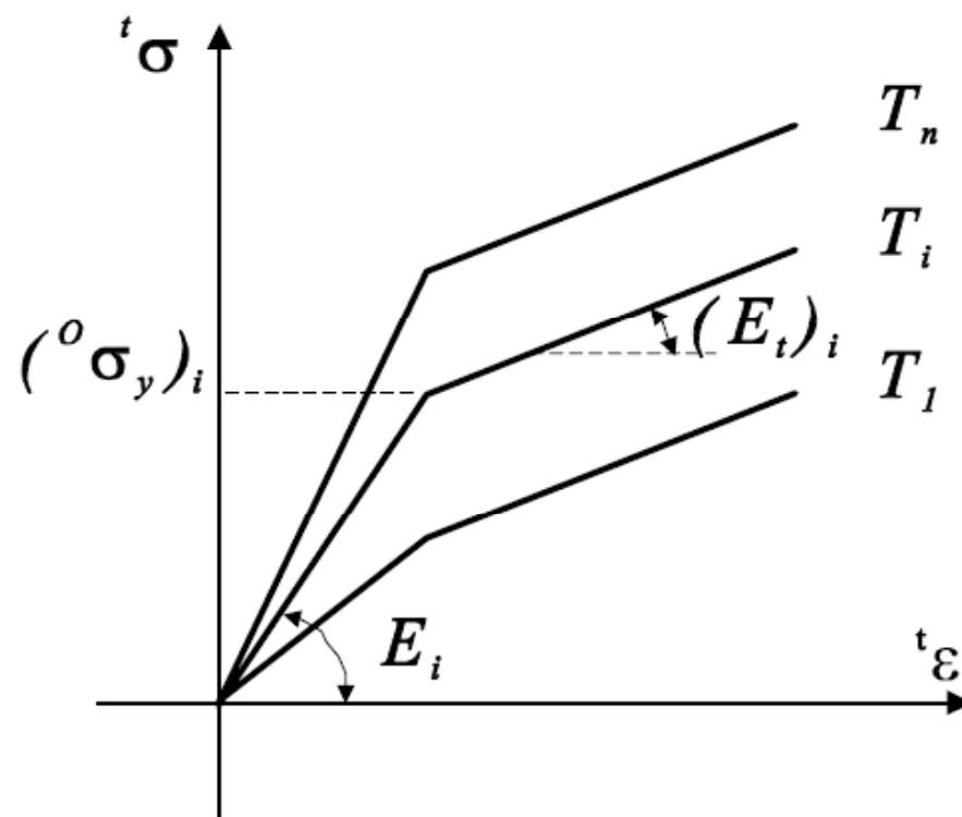
Fig. 5.11. Stress-strain curves at different temperatures,  $T_i$
