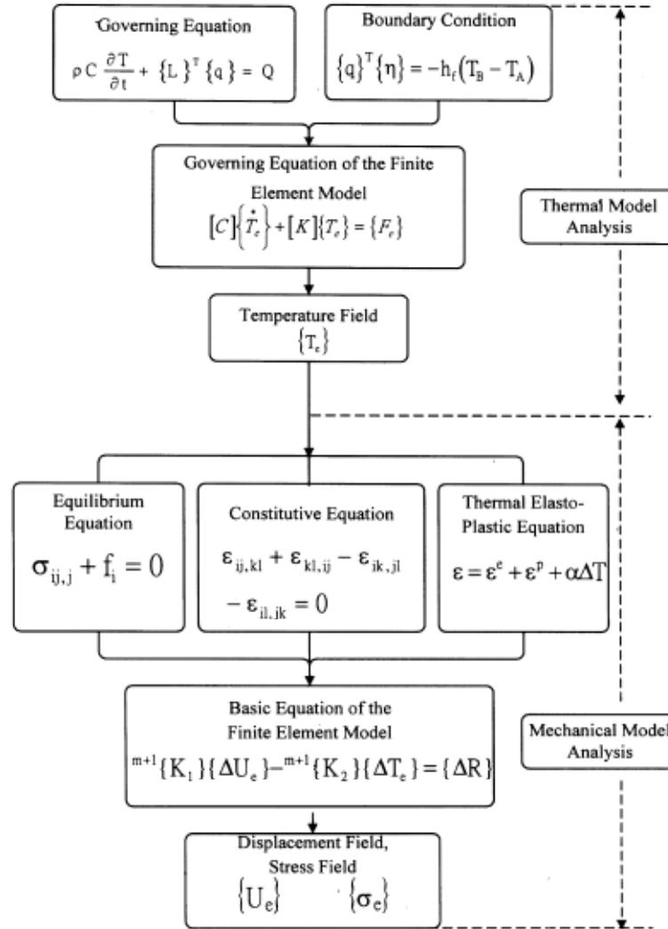
Fig. 1. The analysis procedures for the thermo-mechanical couple field.
