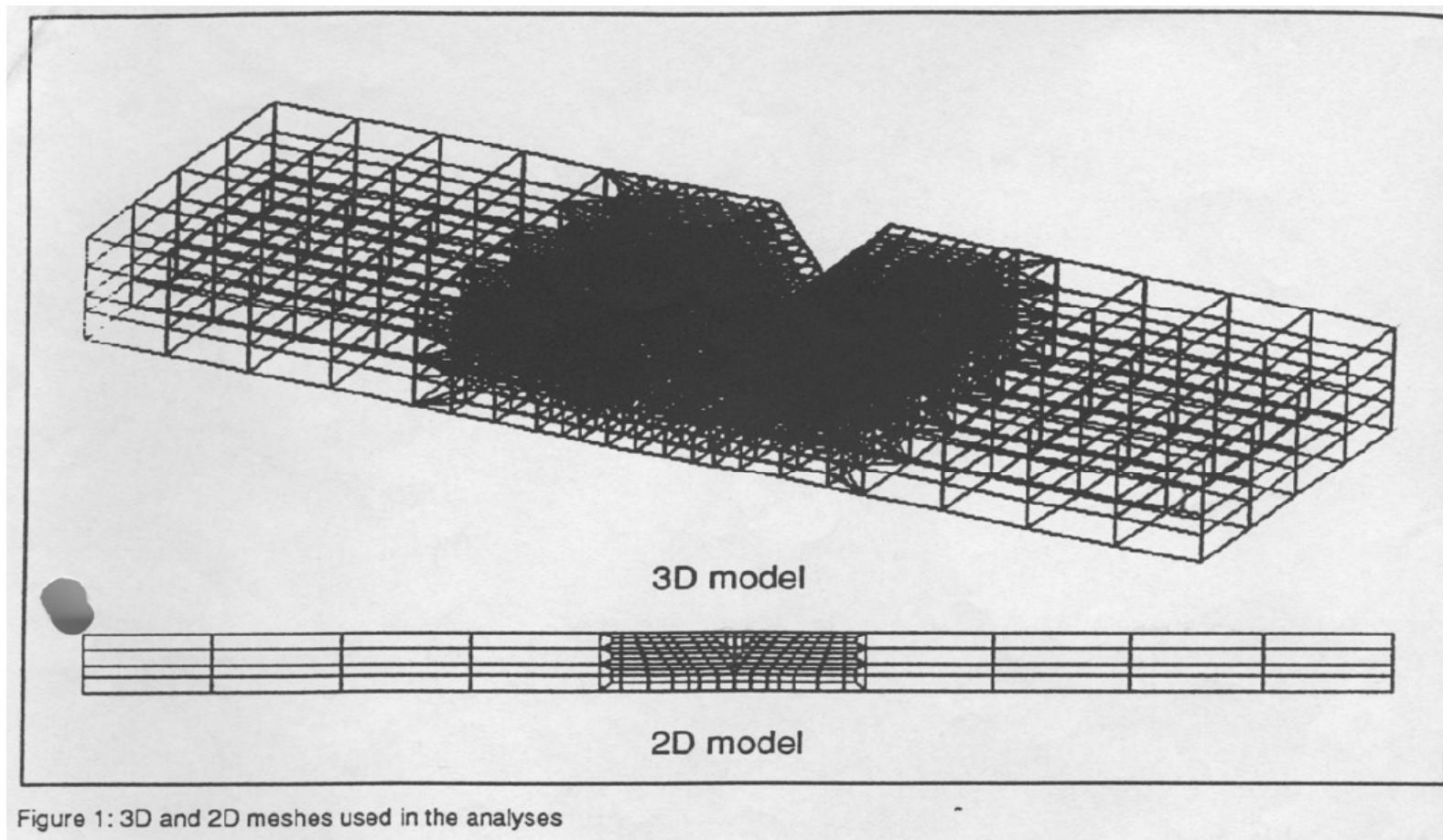
Figure 1: 3D and 2D meshes used in the analyses
