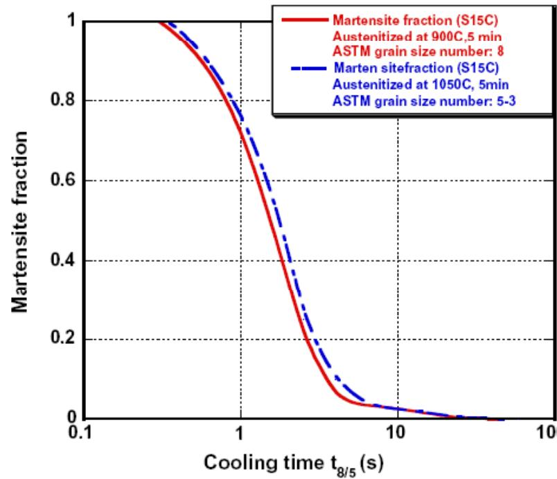
Fig. 5. Martensite fraction as a function of cooling time  $t_{8/5}$  for S15C steel.
