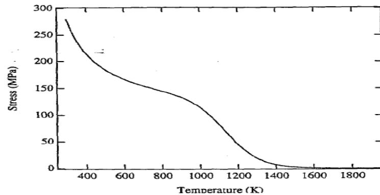
Figure 3. Yield stress of 304L stainless steel used in mechanical finite element analyses as a function of temperature.
