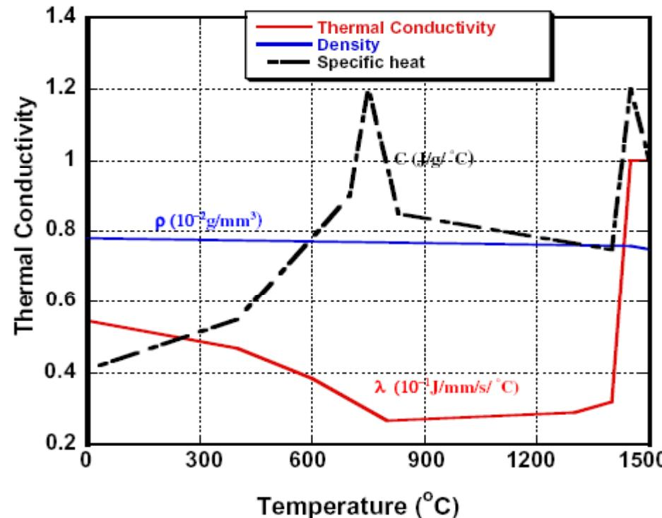
Fig. 3. Temperature-dependent thermal-physical properties.
