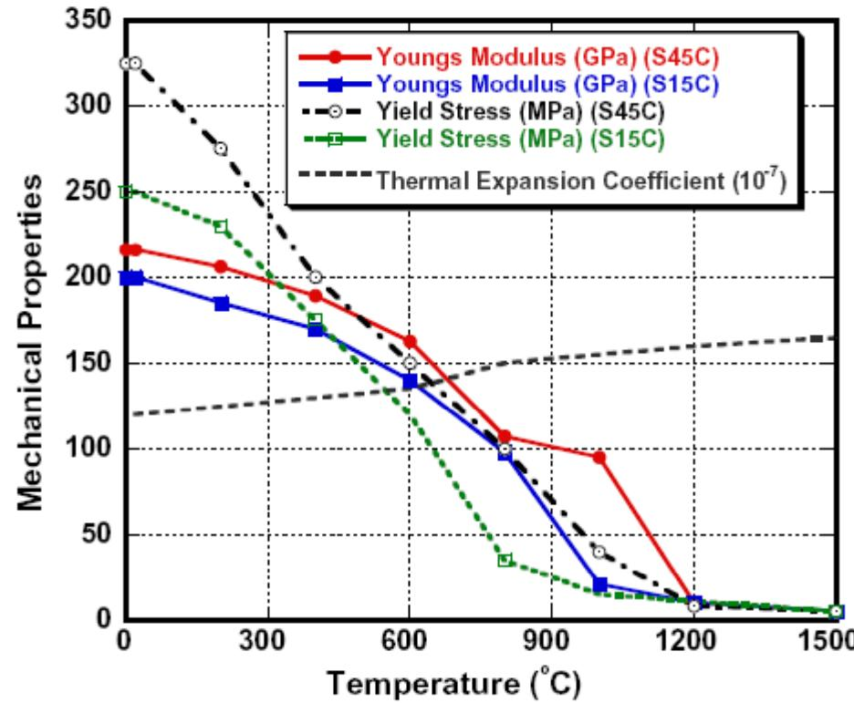
Fig. 7. Temperature-dependent mechanical-physical properties.
