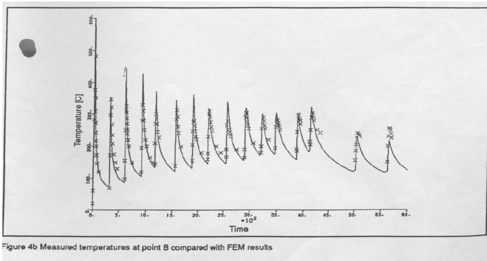
Figure 4b Measured temperatures at point B compared with FEM results
