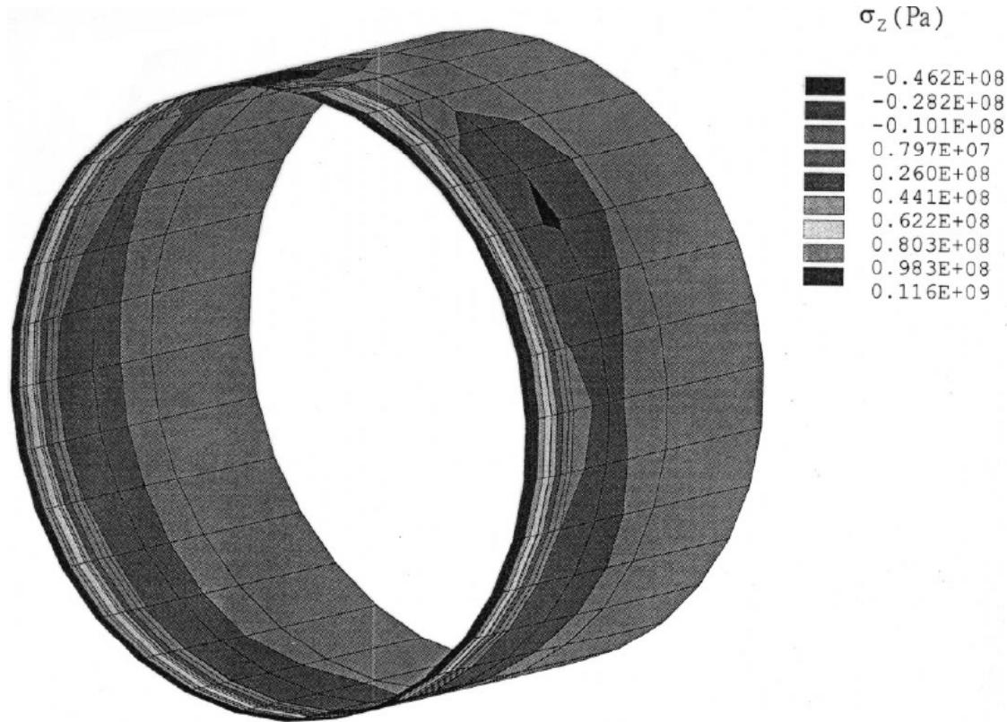
Fig. 9. Contours of residual axial stress at inner surface of 324 mm schedule 10 pipe.
