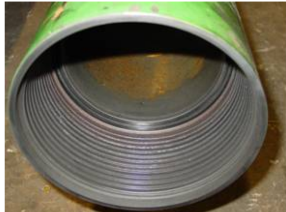
Figure 17 – Visual inspection on Tenaris PJD box side after fatigue test
