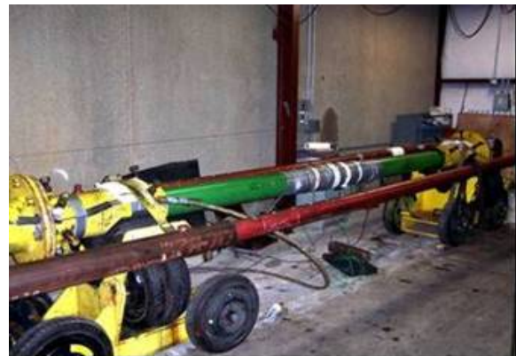
Figure 10 - Resonant fatigue rig set up with an integral upset premium joint (photo by courtesy of Stress Engineering Services Inc.)
