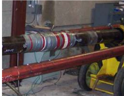
Figure 11 – Leak trap device over the semi-premium joint set up at the resonant rig (photo by courtesy of Stress Engineering Services Inc.)
