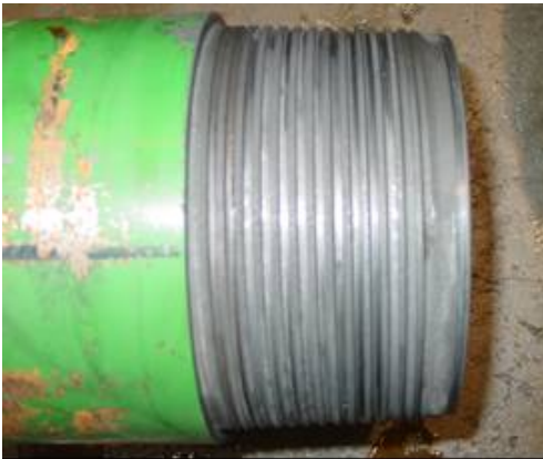
Figure 16 – Visual inspection on Tenaris PJD pin side after fatigue test
