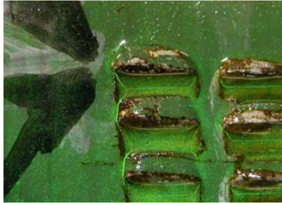
Figure 13 - Crack marks shown by magnetic particles inspection on tong marks
